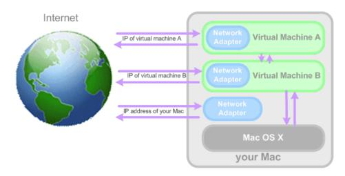
To configure your virtual machine to work in the Bridged Ethernet mode:
