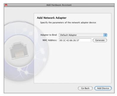
Click the Add Device button to add a new network adapter to the virtual machine.
