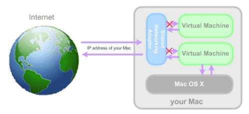
The Shared Networking mode does not require any additional configuration. With this mode enabled, your virtual machine will share whatever network connection your physical computer uses at the moment.
