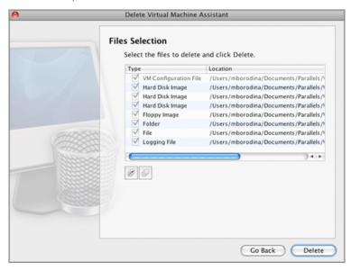
**Note:** Make sure you are not going to delete the virtual hard disk that is also used by other virtual machines.
